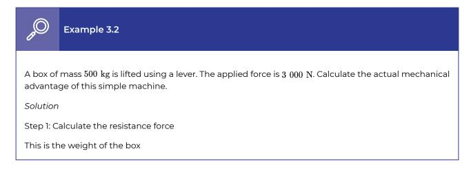
$F_g = mg$   $= 500 \ge 9.8$   $= 4 \ 900 \ \text{N}$ Step 2: Write the formula for actual mechanical advantage  $AMA = \frac{F_r}{F_e}$ Step 3: Substitute the given values  $AMA = \frac{4 \ 900}{3 \ 000}$ Step 4: Write the answer AMA = 1.63
