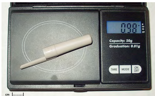
Figure 1.20 Whereas a mechanical balance may only read the mass of an object to the nearest tenth of a gram, some digital scales can measure the mass of an object up to the nearest thousandth of a gram. As in other measuring devices, the precision of a scale is limited to the last measured figures. This is the hundredths place in the scale pictured here. (Splarka, Wikimedia Commons)
