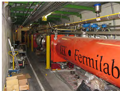
Figure 1.6 Particle colliders such as the Large Hadron Collider in Switzerland or Fermilab in the United States (pictured here), have long tunnels that allows subatomic particles to be accelerated to near light speed. (Andrius.v)
