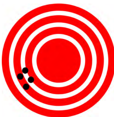
Figure 1.22 In this figure, the dots are concentrated close to one another, indicating high precision, but they are rather far away from the actual location of the restaurant, indicating low accuracy. (Dark Evil)
