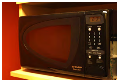
Figure 1.7 Why can't you put metal in the microwave? Microwaves are high-energy radiation that increases the movement of electrons in
